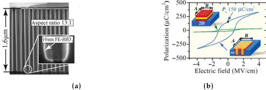
Figure 2.6: (a) TEM imaging and (b) P-E relation of a 3-D capacitor TiN/HfO 2 /TiN. A and B are the dimensions of the projected area which can be computed as A \cdot B [46].
