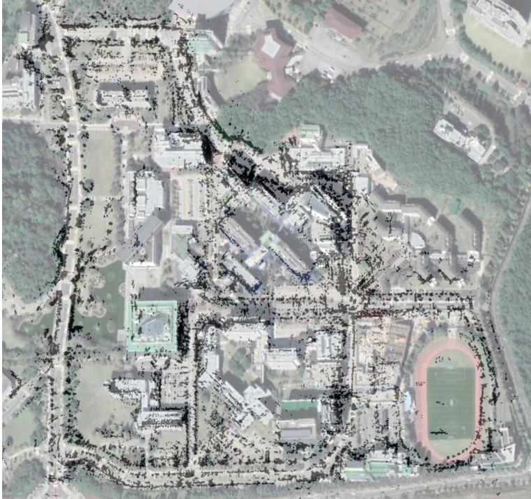
Figure 7.4: Map of Sequence KAIST03 of the MulRan dataset [182], built by the proposed algorithm, RadART-SLAM, overlaid on the corresponding area visible in Google Earth.
