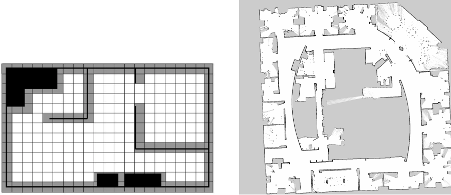
Figure 2.11: On the left, 2D occupancy grid representation of a map; on the right, large scale 2D reconstructed map in an occupancy grid.
