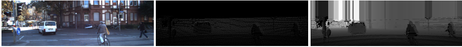
Figure 4.5: From left to right, RGB image, sparse range image obtained through LiDAR-to-camera projection and enhanced range image, from city Sequence 05 of the KITTI raw dataset [144]. The enhancement is achieved through simple bilinear filtering.
