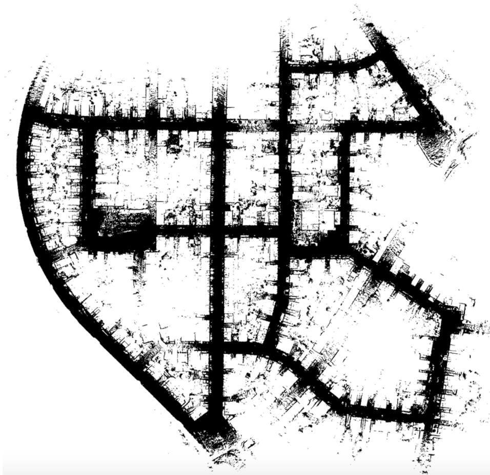
Figure 3.8: Reconstructed 3D map of Sequence 00 of the KITTI odometry dataset [143], obtained with the developed system, ART-SLAM [1].
