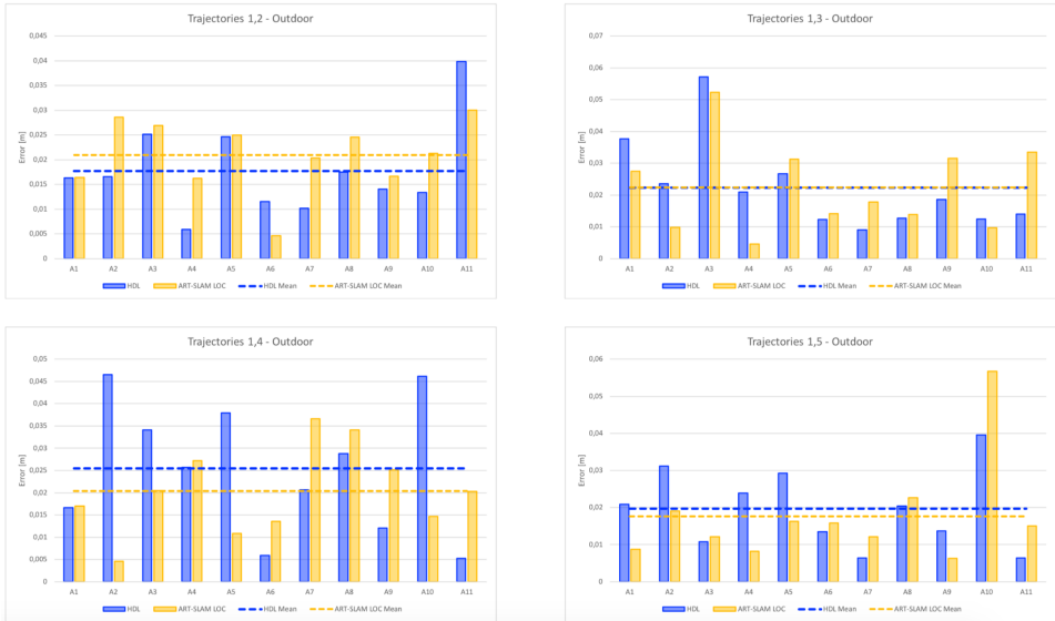
Figure 3.16: Translation re-localization errors of the outdoor experiment, using HDL [28] and ART-SLAM [1]. The accuracy of both systems is noticeable.
