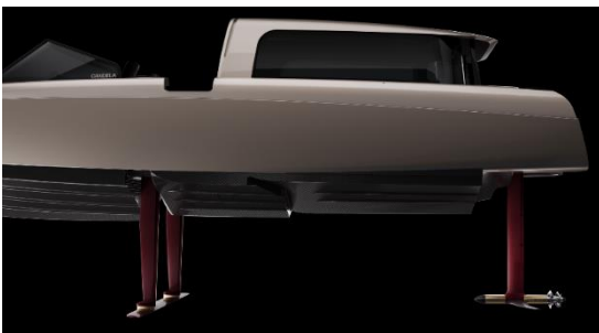
Fig. 2.18 d - Foiling mode, which allows high efficiency navigation and to reach longer ranges.
