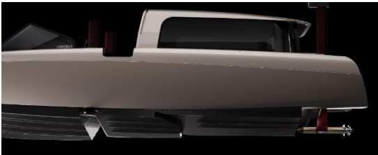
Fig. 2.18 b - Shallow mode, for low speeds and for navigating lower channels.
