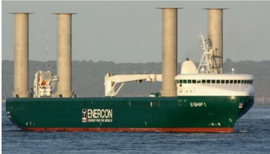
Fig. 1.11 - Flettner rotor installed on E-ship 1 project.
