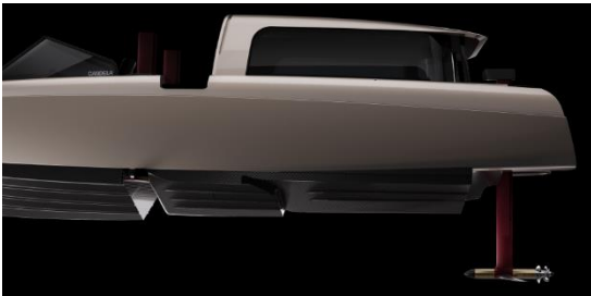
Fig. 2.18 c - Planing mode, for navigation at cruising speed.
