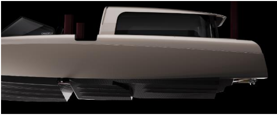
Fig. 2.18 a - Harbor mode, in which the foils are fully retracted.
