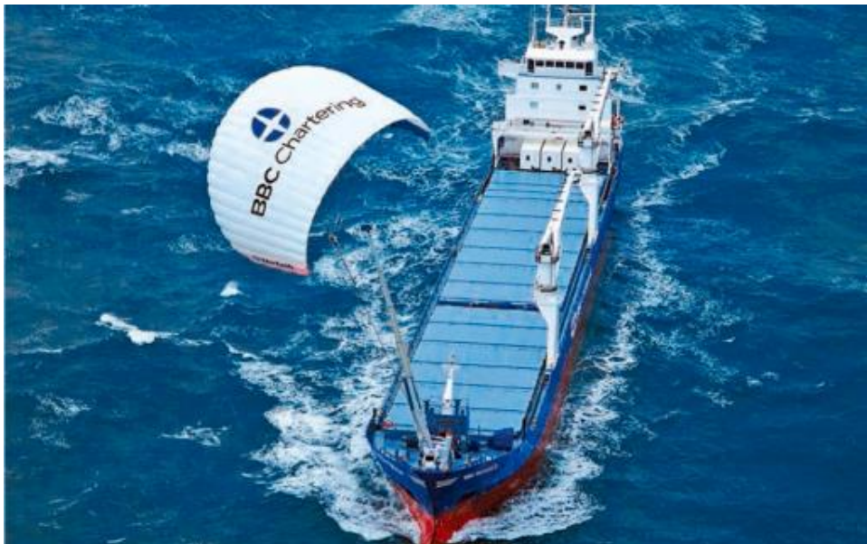
Fig. 1.12 - Kite solution installed on a cargo ship.
