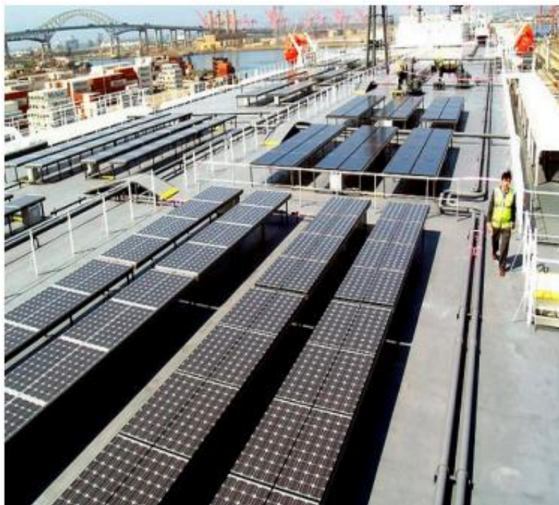
Fig. 1.10 - Solar panels installed on a cargo ship.
