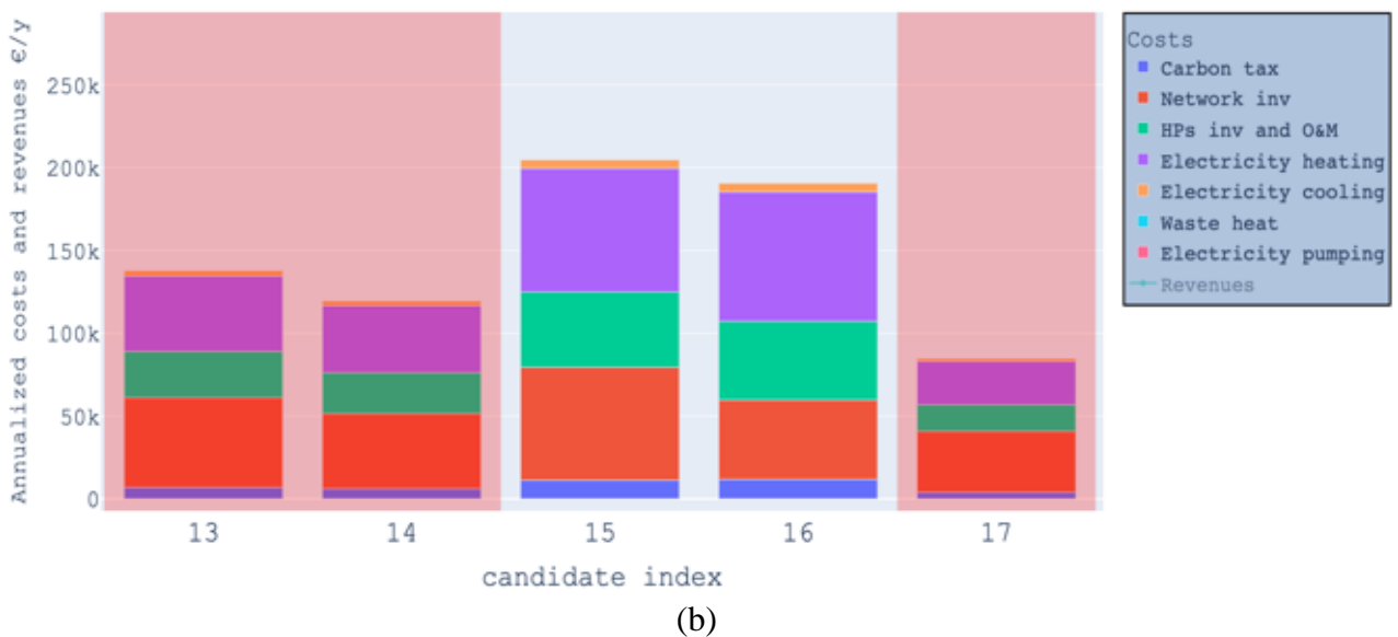
Figure 57. (a) A 50% increase in electricity prices shows how the NT-DHC solution outperforms the benchmark technologies. (b) The increase in the energy price and its impact on the NT-DHC solution.
