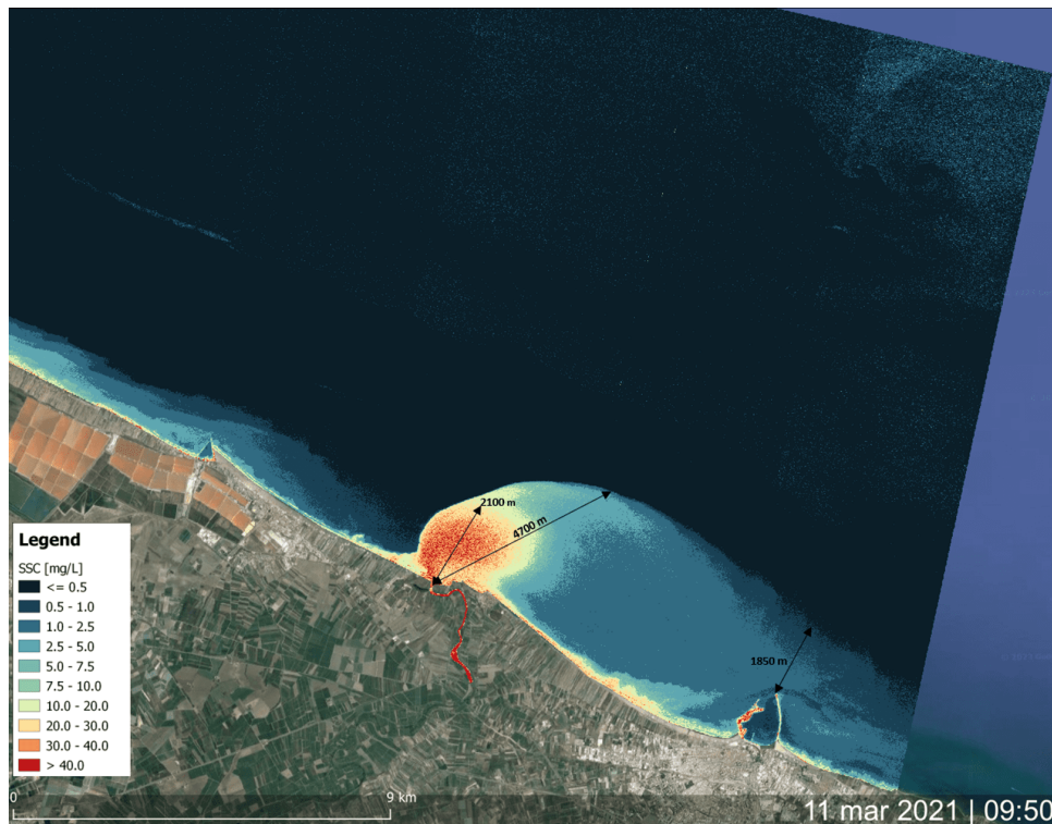
(a) Suspended sediment concentration on March 11, 2021, calculated with the formula calibrated in [Zhang et al., 2014].
