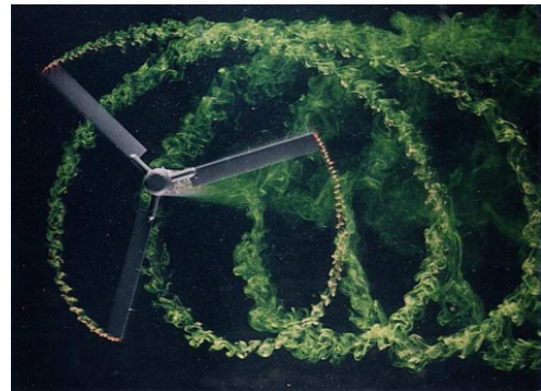
(b) Wake visualization of a three-bladed rotor in forward flight
