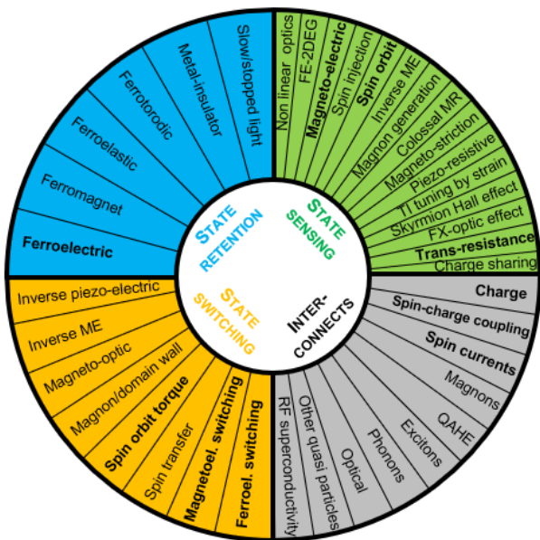
Figure 1: Beyond-CMOS "Wheel of technologies" for state retention, state sensing, state switching and interconnects.
