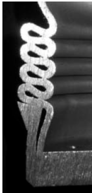
Figure 1.9: Collapse mechanism in an aluminum alloy absorber [2].
