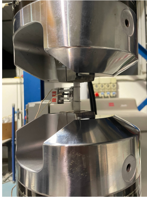
Figure 3.16: Positioned specimen with extensometer mounted.
