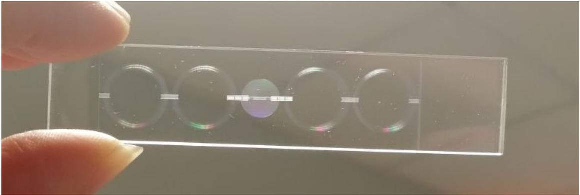
Figure 5.12. Picture of a fused silica slab irradiated with the geometry of the differential pumping chip.
