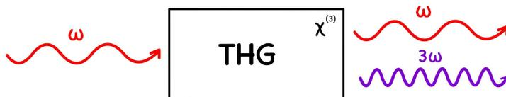
Figure 2.3. Schematic representation of Third Harmonic Generation via  $\chi^{(3)}$  materials.
