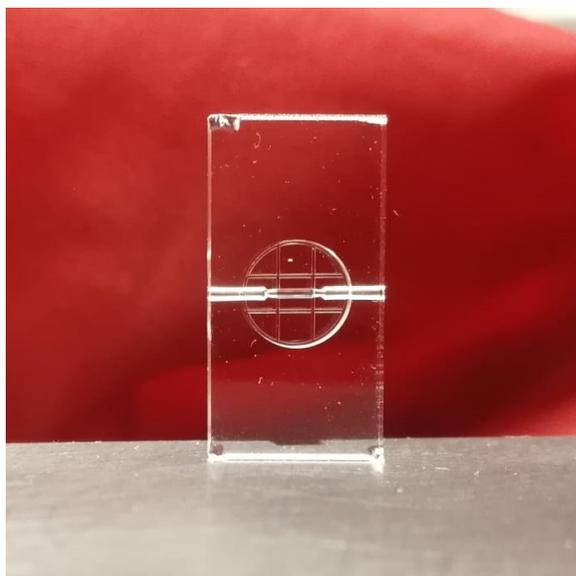
Figure 5.10. Picture of the THG cell fabricated in a fused silica slab.
