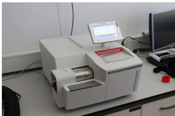
Figure 2.8: Mettler Toledo TGA/DSC 3+ device.
