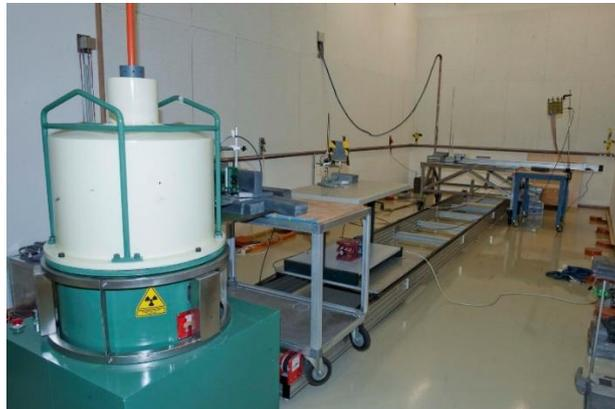
Figure 2.10: Co60 irradiation facility at ESA ESTEC [68].
