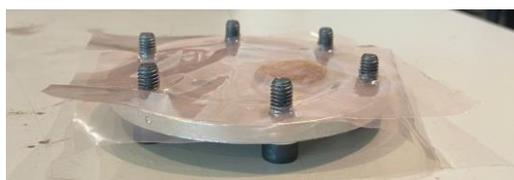
(b) Upper sealing ring with specimen
