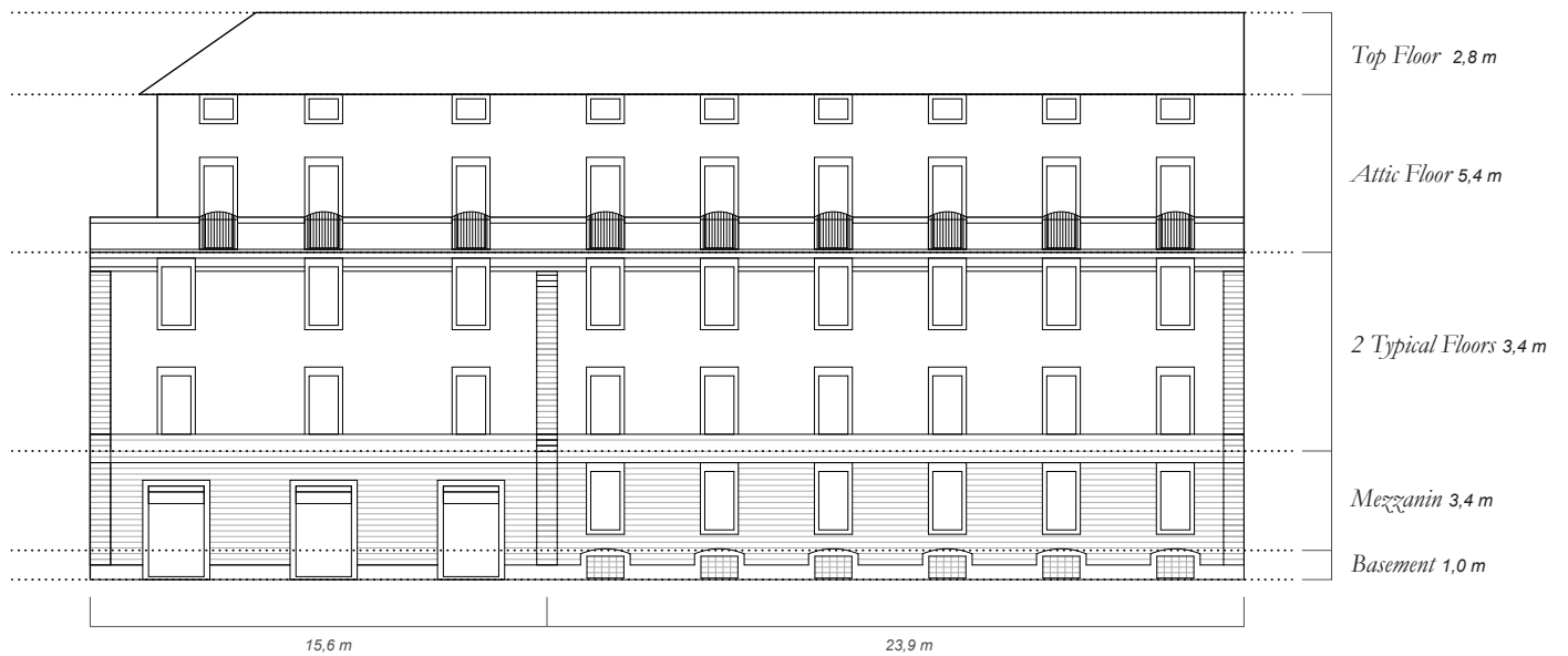
Building Facade Elevation - Out of Scale
