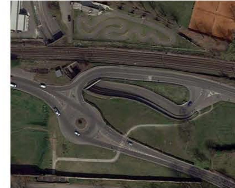
Existing roundabout with three exits (Via XXI Aprile, Via Cardinale Maculani). A tunnel for vehicular circulation is crossing underneath the railways to reach to tower part and the water front..
