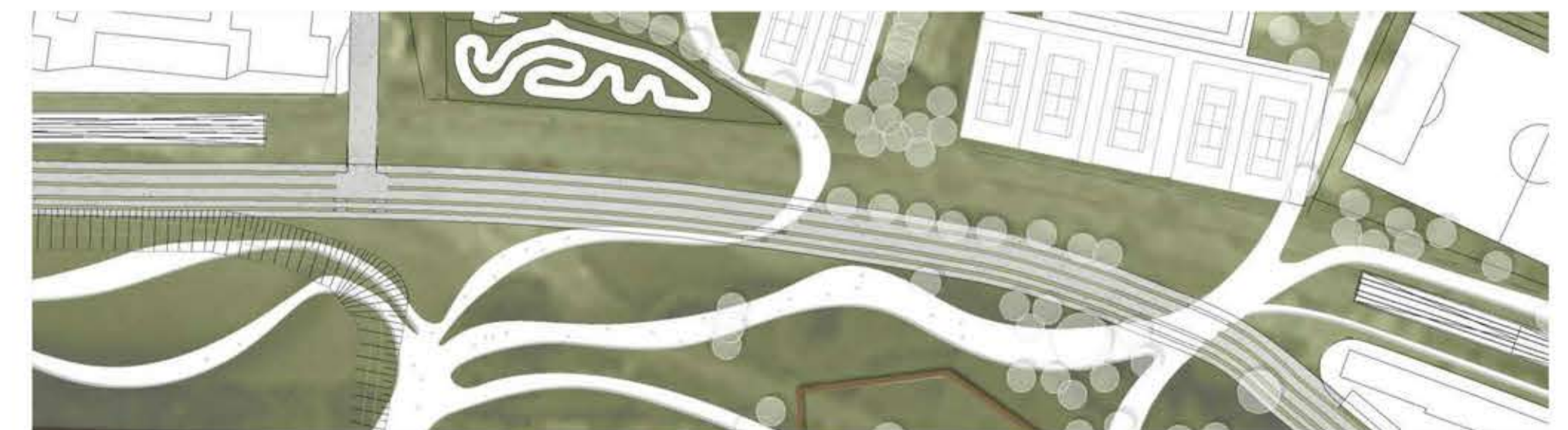
A new tunnel was added between the two selected points. 1,5% slopes from both sides with a length of 450 meters were added to reach the clearance level for the trains. Slopes are left uncovered.
