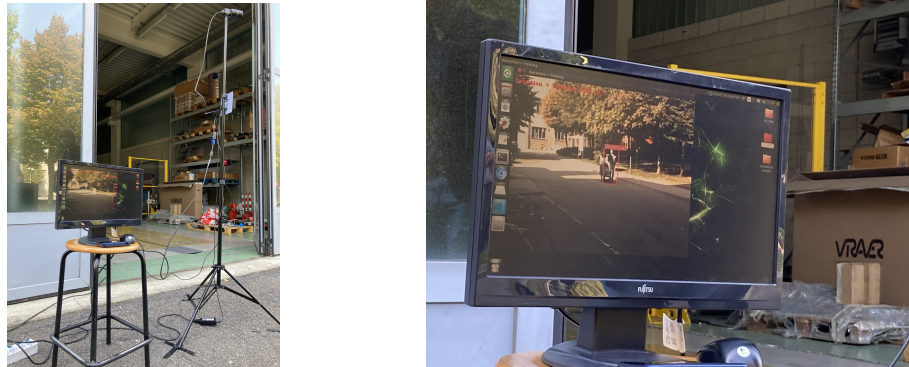
Figure 6.9: Camera Setup at the location of pedestrian crossing that could relay I2V communication over a 5G network.
