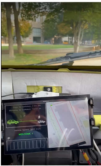
(a) Pedestrian is invisible, Vehicle speed while negotiating the turn is 2.02 m/s, Visual Warning is Green, TTC is 7.54 seconds, Distance to collision is 14.47 m.
