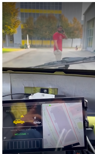
(b) Pedestrian is visible, Vehicle speed is 2.03 m/s Visual Warning is Amber, TTC is 2.27 seconds, Distance to collision is 4.6 m.
