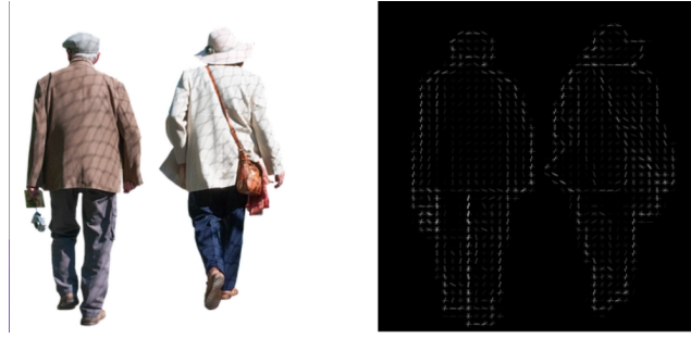
Figure 10: Initial image and intermediate HOG features representation. Source: [27]
