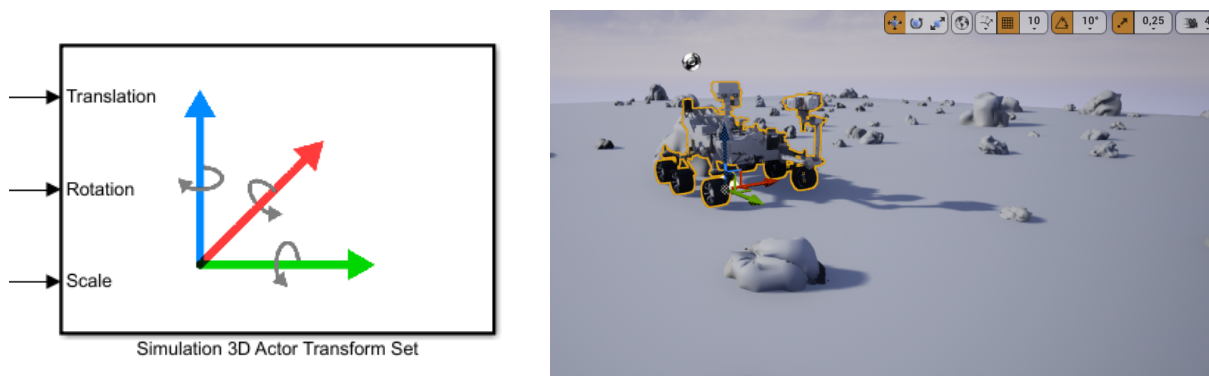
Figure 2.5: Simulation 3D Actor Transform Set block and Unreal Engine actor
