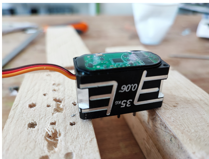
Figure 3.9: Waterproofing of the servomotors with the dielectric gel
