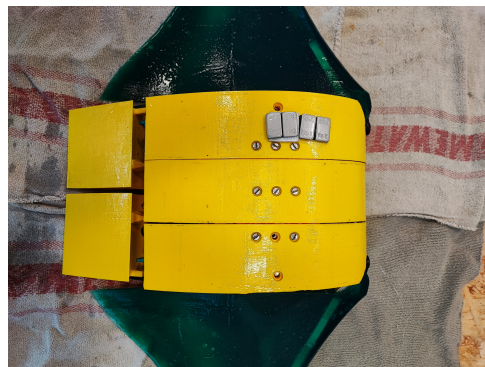
(b) Ballast on the external structure
