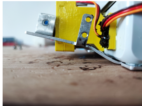
(b) Rear part of the chassis that was bent to be no longer horizontal
