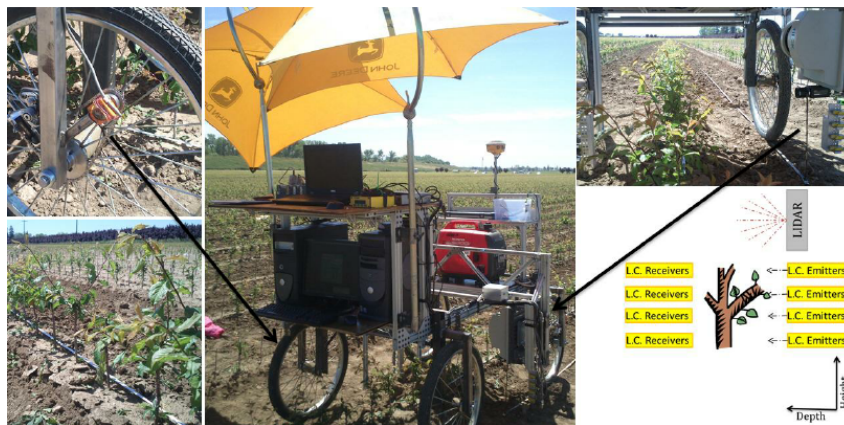
Figure 1.2: The cart used by [5] with highlights of the mounted sensors. On the top left, the encoder coupled with a timing chain, mounted on the wheel. On bottom left, the tree stem detection. On the right the arrangement of the LiDAR and the light curtain. (taken from [5])
