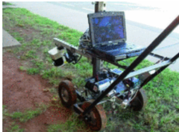
Figure 1.5: The custom cart built in [22]. The LiDAR is placed on the left of the cart and inclined of 20^\circ with respect to the ground.
