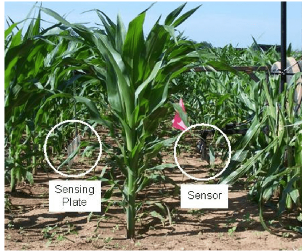
Figure 1.1: Sensor and reflective plate placement during field testing (taken from [9])
