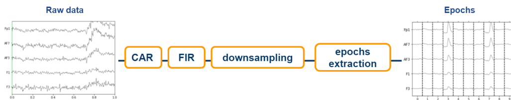
Figure 2.2: Data preprocessing pipeline. From raw data common average is subtracted (CAR), then a FIR filter is applied to extract the band between 1 and 10 Hz, data are downsampled to 64 Hz and finally epochs are extracted.
