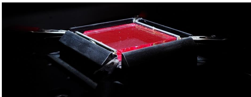
Figure 3.44 – No mask configuration for PV tests in LSC devices.
