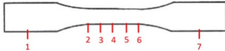
Figure 38 - Thickness measurement points
