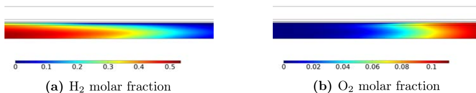
Figure 3.10 – Simulated concentration of hydrogen (left) and oxygen (right) during the start-up process. The images are taken at t = 0.14\text{ s} and both represent the same relevant portion of the domain, from x = 11\text{ mm} to x = 24\text{ mm} .
