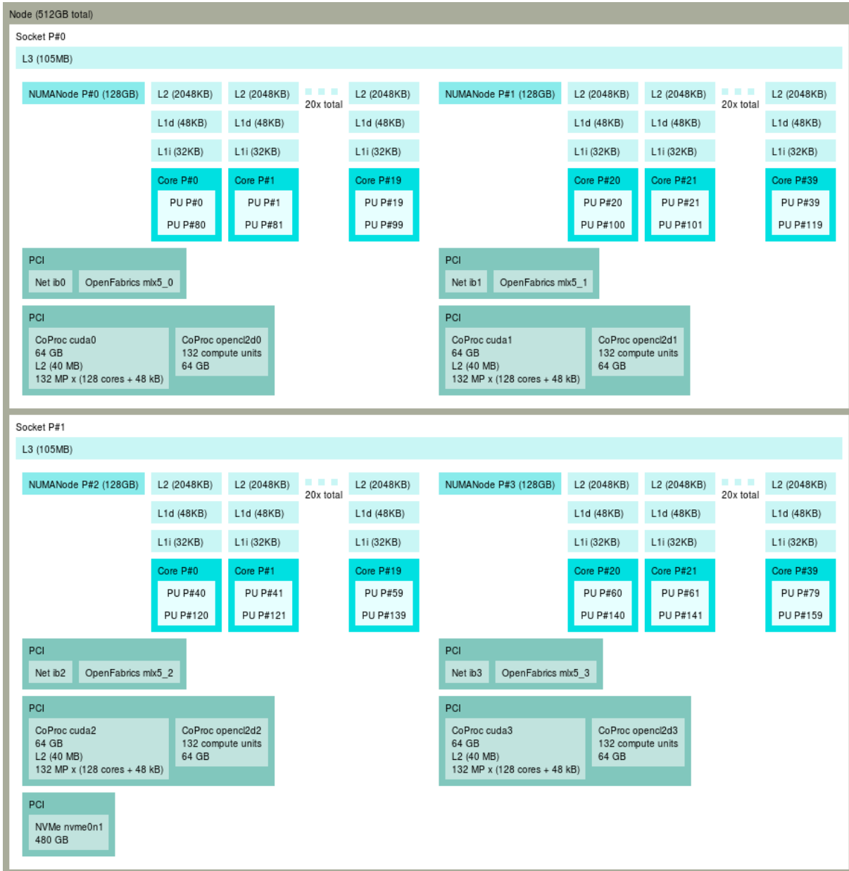
Figure 4.1 MareNostrum 5 ACC node topology. Hardware-locality map ( hwloc/lstopo ) of a MareNostrum 5 Accelerated Partition (ACC) compute node used for the experimental runs. The node integrates two Intel Xeon Platinum 8460Y+ sockets (40 cores per socket, 80 cores total) and 512 GiB of DDR5 memory exposed as four NUMA domains (128 GiB each). Each core exposes private caches (L1i 32 KiB, L1d 48 KiB, L2 2 MiB), while each socket provides a shared L3 cache of 105 MiB. The PCIe/I/O layout includes four NVIDIA H100 GPUs (cuda0–cuda3, 64 GB HBM per device; 132 SMs and 40 MiB L2 per device as reported by the topology tool) and four ConnectX-7 NDR200 InfiniBand HCAs (mlx5_0–mlx5_3 mapped to ib0–ib3). A local NVMe device ( nvme0n1 , 480 GB) is available for node-local scratch. Taken from [3].
