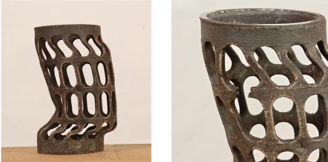
Figure 4.24 Right: deformed structure at failure; left: close-up view of crack. (Configuration A)
