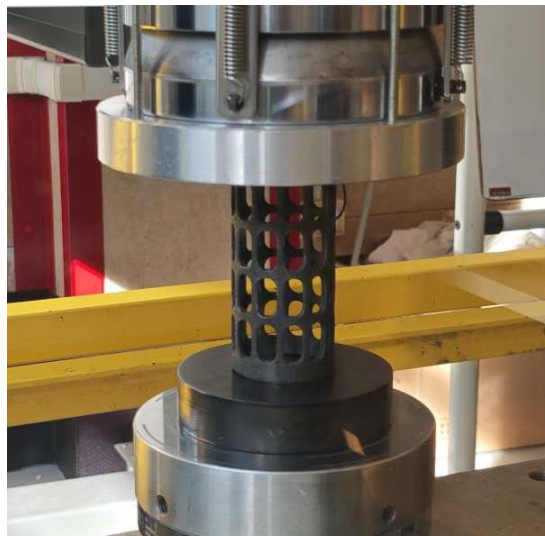
Figure 4.21 Real compression test setup.
