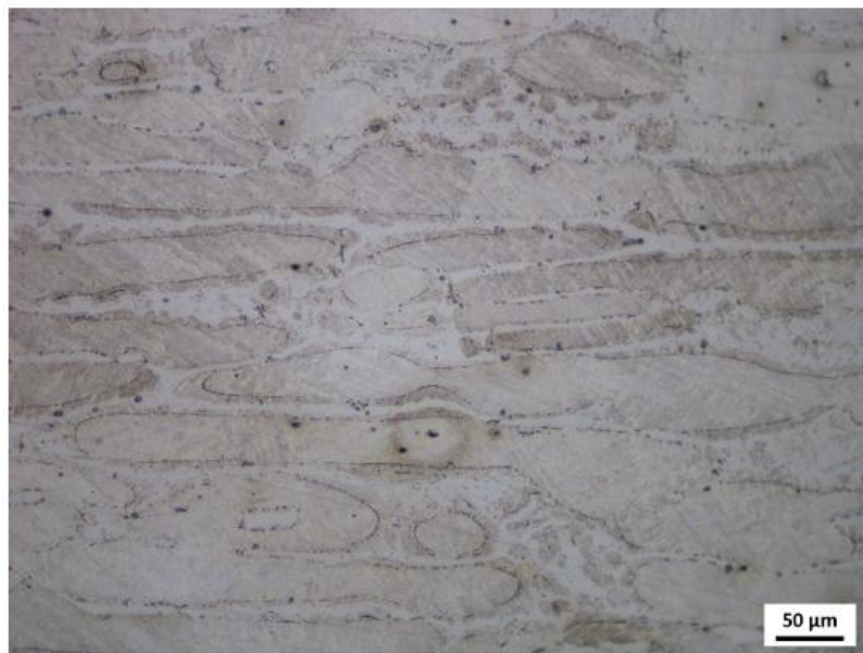
Figure 3.2 Hot rolled and solubilized Alloy 2 microstructure image taken with optical microscope.
