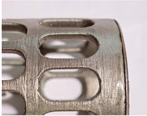
Figure 4.17 Surface quality of casting product.
