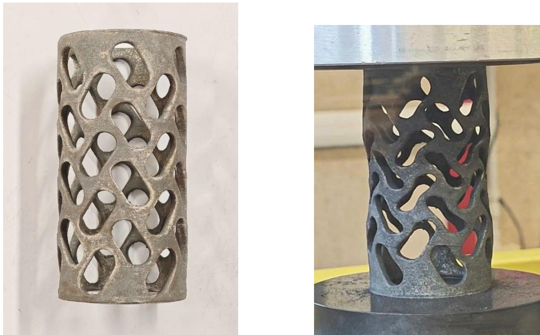
Figure 4.28 Deformed structure under compression: 5mm displacement (left); 12mm displacement (right). (Configuration C)
