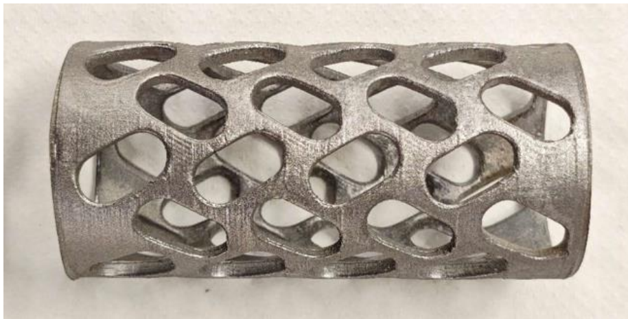
Figure 4.20 As cast bioinspired lattice structures (Configuration C)
