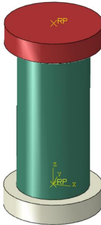
Figure 2.16 Assembly of the compression test on Abaqus: Red part is the head (moving plate), white part is the base (fixed plate) and the green one is the sample to be tested. Both plates are discrete rigid solid with reference point.
