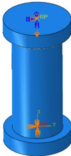
Figure 2.18 Boundary conditions applied at the reference points of the rigid bodies.
