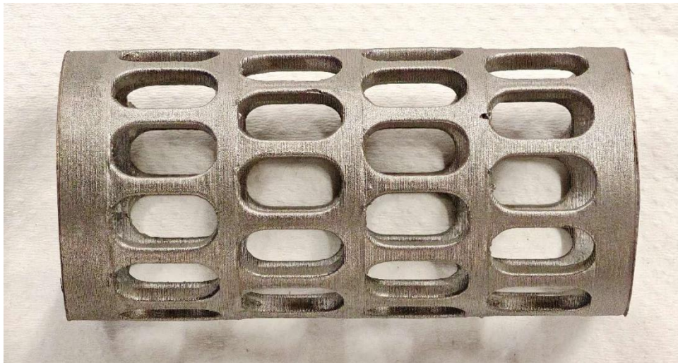
Figure 4.19 As cast bioinspired lattice structures (Configuration B)
