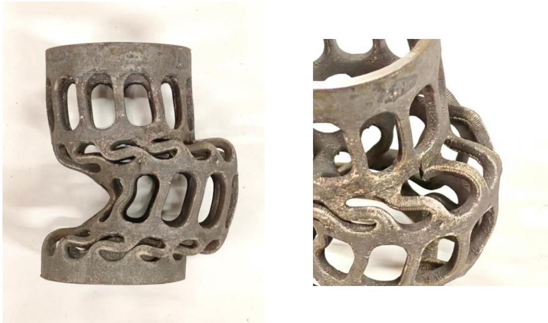
Figure 4.27 Right: deformed structure at failure; left: close-up view of crack. (Configuration B)
