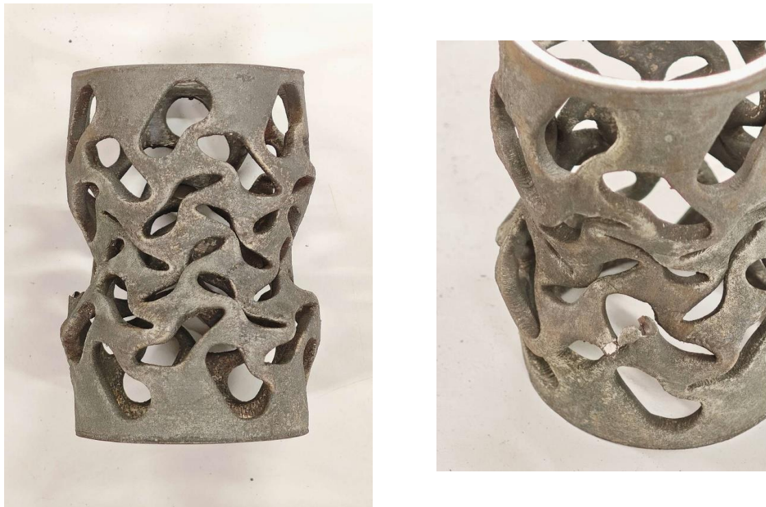
Figure 4.30 Right: deformed structure at failure; left: close-up view of crack. (Configuration C)
