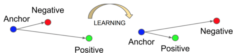
Figure 2.10: Visualization of triplet loss goal, reduce the distance of an anchor to the positive example and increase the distance to the negative one.
