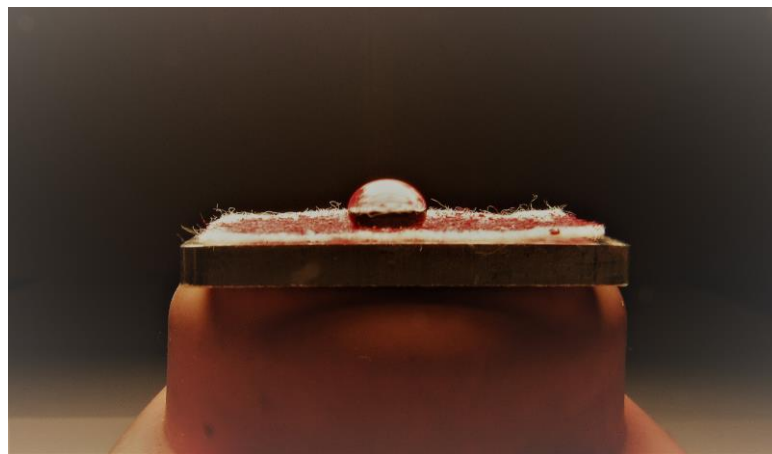
Figure 3.2 - Picture of a drop deposited on the wipe coated with a thin layer of nail polish. Sample showed an hydrophobic behavior.
