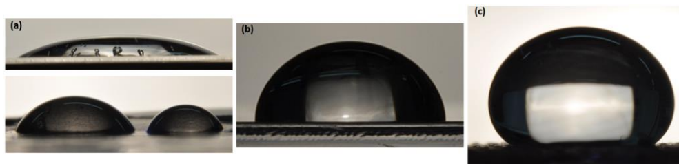
Figure 1.2 - Examples of contact angles formed by sessile liquid drops on an horizontal homogeneous solid surface: (a) hydrophilic surface/wetting drop with a \theta_c < 90^\circ (b) threshold situation with \theta_c = 90^\circ (c) hydrophobic surface/non-wetting drop with \theta_c > 90^\circ (in this last case the surface is not smooth). Picture taken from [41].
