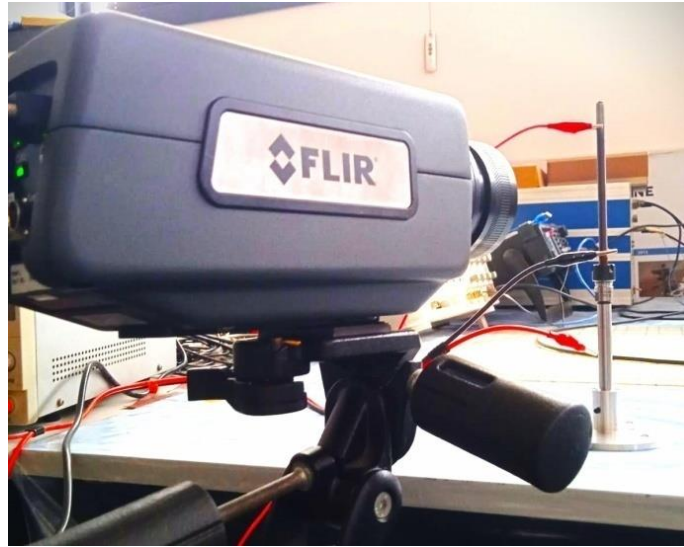
Figure 3.18 Thermocamera and tube in vertical configuration
