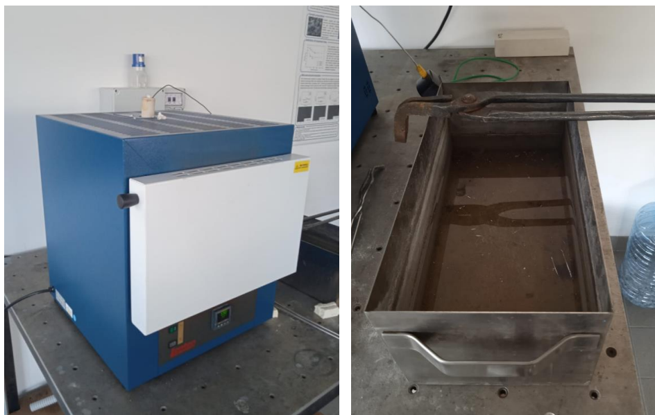
Figure 2.4 Lenton furnace and quenching water
