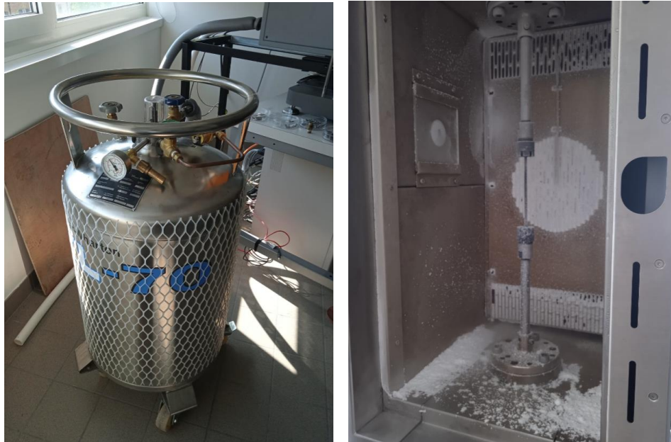
Figure 2.7 The use of Nitrogen was required to reach low temperatures
