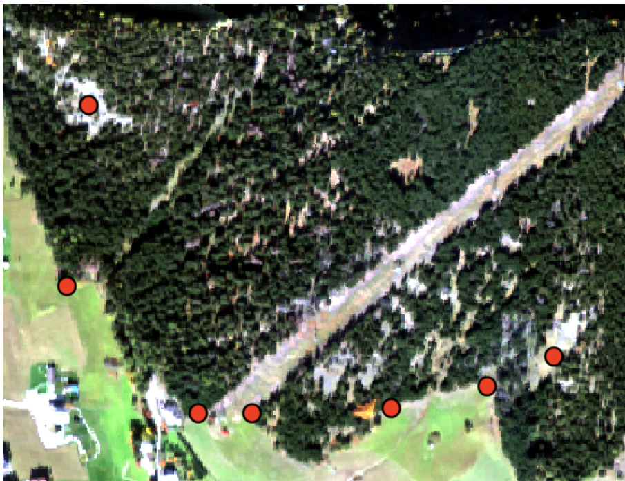
Figure 4.2: The set of 7 double points selected for image coregistration on asiaFENIX image
