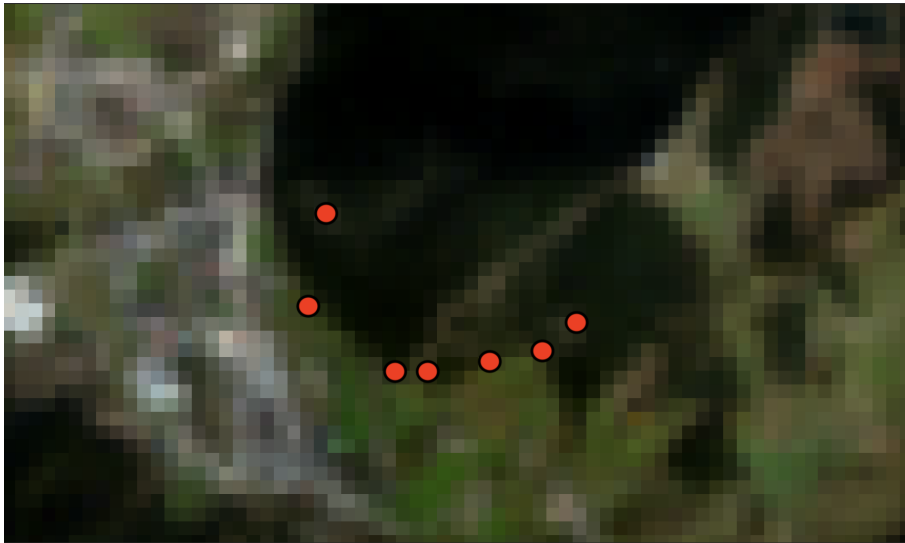
Figure 4.1: The set of 7 tie points selected for image coregistration on PRISMA image
