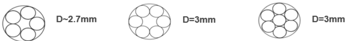
Figure 2.9: Scheme of the arrangements and respective total diameters of a OPTIMEDIA 1 bundle.
