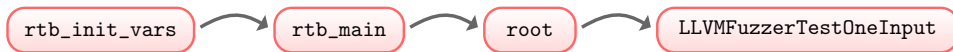
Figure 3.3: A representation of the transition back to root that occurs when initializing fuzzing. The program is let run till, for instance, the end of rtb_init_vars , which is an isolated function that is supposed to be executed for starting up the program correctly. Once completed, it returns to the caller, rtb_main . Here, instead of continuing the normal execution, the control is transferred back to root , which ultimately ends the execution of the guest program (leaving it in a valid state) and returns to LLVMFuzzerTestOneInput.
