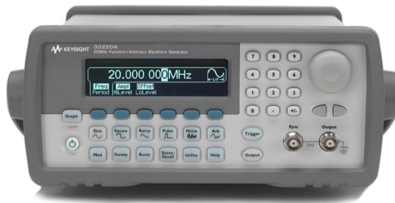
Figure 7: Keysight 33220A, 20 MHz Functional/Arbitrary Waveform Generator
