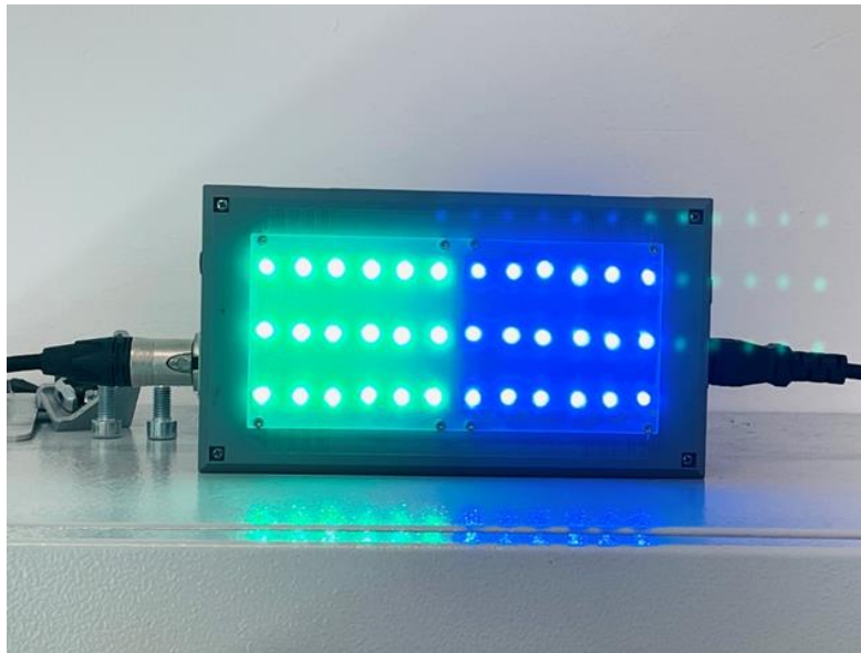
Figure 12: PVT test device, with blue and green diodes
