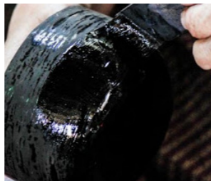
The black lacquer is applying on wooden surface, makes it smooth and shiny.
