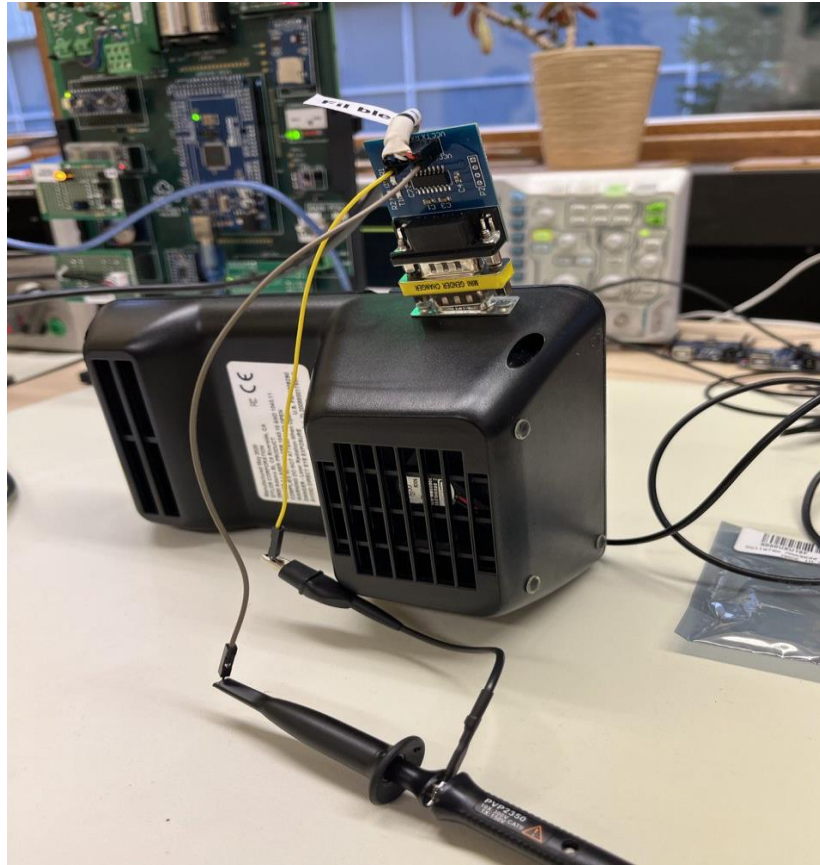
Figure 6 Dylos connection to the PCB
