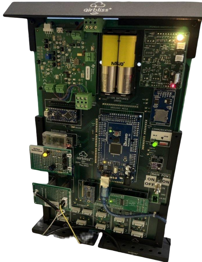
Figure 14: Assembled PCB with Integrated Components for System Functionality Testing
