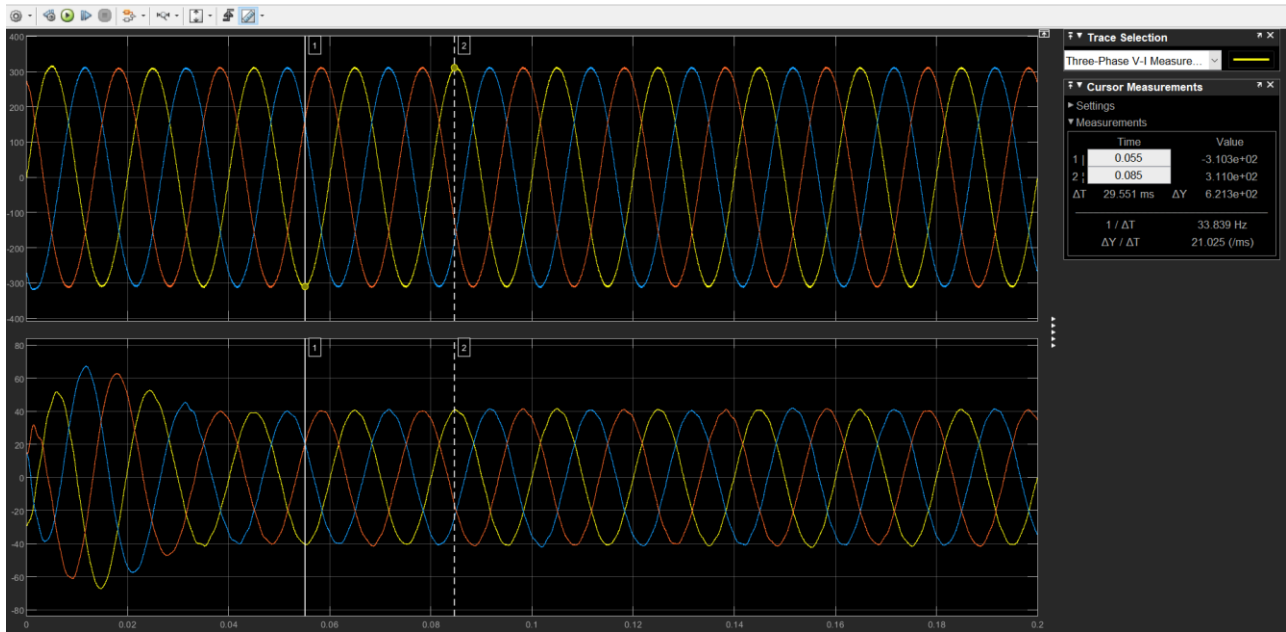
Figure 55-Inverter 1 output voltage and current
