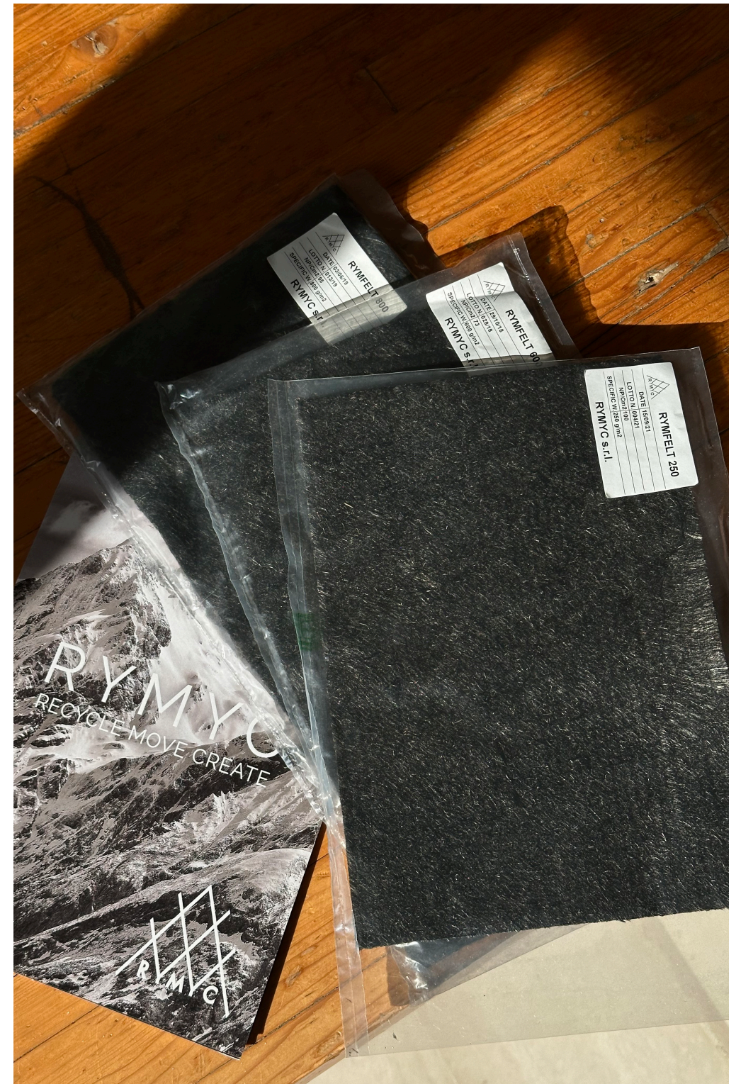
Figure 27: Rymfelt carbon fibre nonwoven samples with increasing areal weight, 250 g/m 2 , 600 g/m 2 , and 800 g/m 2
