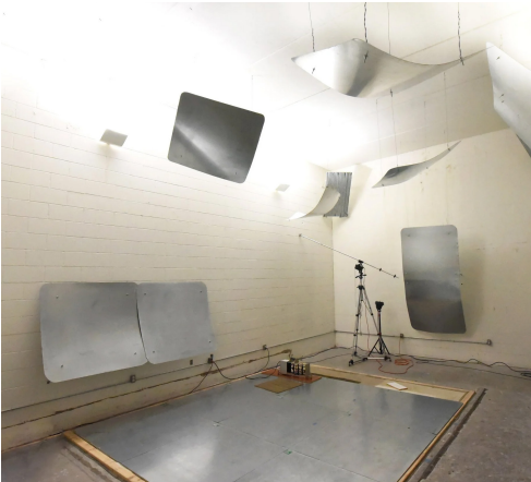
Figure 15: reverberation room method setup
