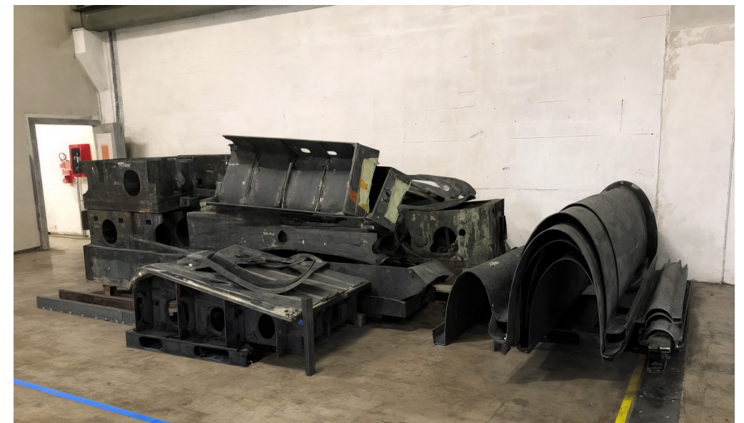
Figure 25: Incoming carbon-fibre composite waste stream used as feedstock for Rymfelt recycling.
