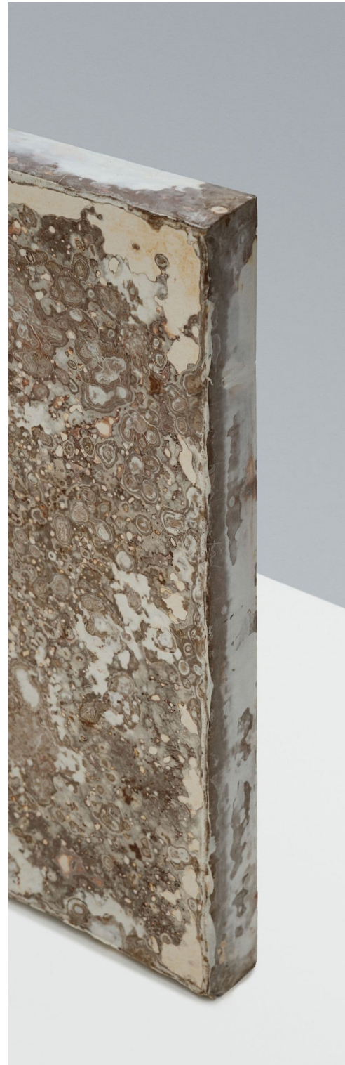
Figure 23: mycelium based panel from Myceen
