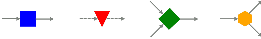
Figure 2.1: Visual classification of the industrial processing nodes. From left to right: Machine (0), Buffer (1), Assembly (2), and Disassembly (3).
