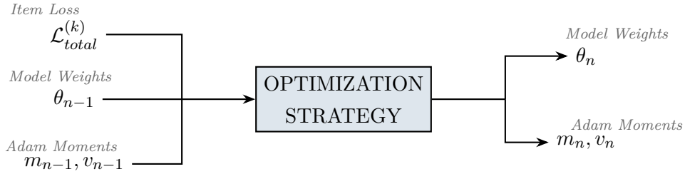
Figure 3.9: Input-output architecture of the Optimization Strategy block as integrated within the Diffusion Training Framework.
