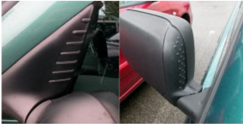
Figure 11: Vortex generator to avoid tonal noise in the area of two exterior mirrors of production vehicles [9].
