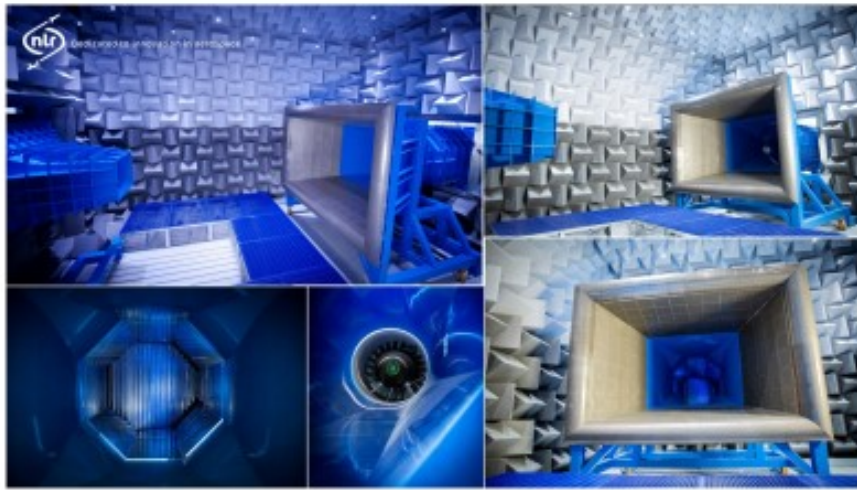
Figure 3: Royal NLR Anechoic wind tunnel which shows a particular use sound absorbing materials [22].
