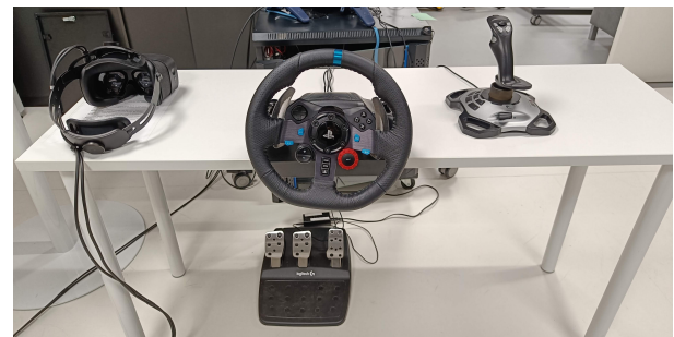
Figure 8: The second iteration introduced a Logitech G29 steering wheel to drive the reach stacker. The Extreme 3D joystick was mapped to control the boom and spreader.
