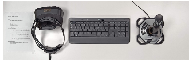
Figure 3: The physical devices used for the first iteration include a Varjo XR-3 HMD, a keyboard and a Logitech Extreme 3D joystick.
