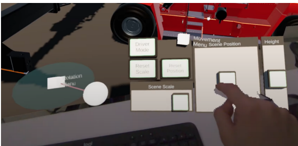
Figure 4: Virtual interactions include a rotation menu to rotate the virtual scene around the user, and a movement menu with sliders to change the scale of the virtual scene and allow free movement inside the scene.
