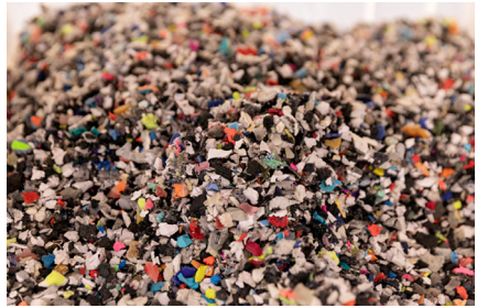
Figure 55. The mixture of rubber, foam, fiber, leather and textiles is separated and ground into various particles.
