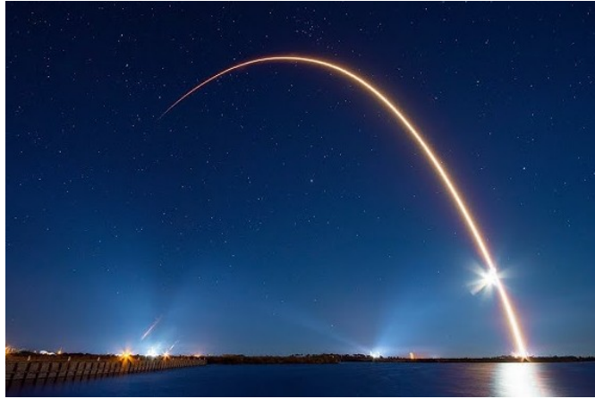
Figure 2.13: Trajectory during gravity turn. (Source: SpaceX)
