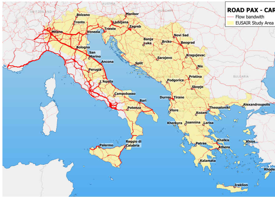
Figure 3.1: CAR Passenger Transport - Flow bandwidth [PAX/DAY]
