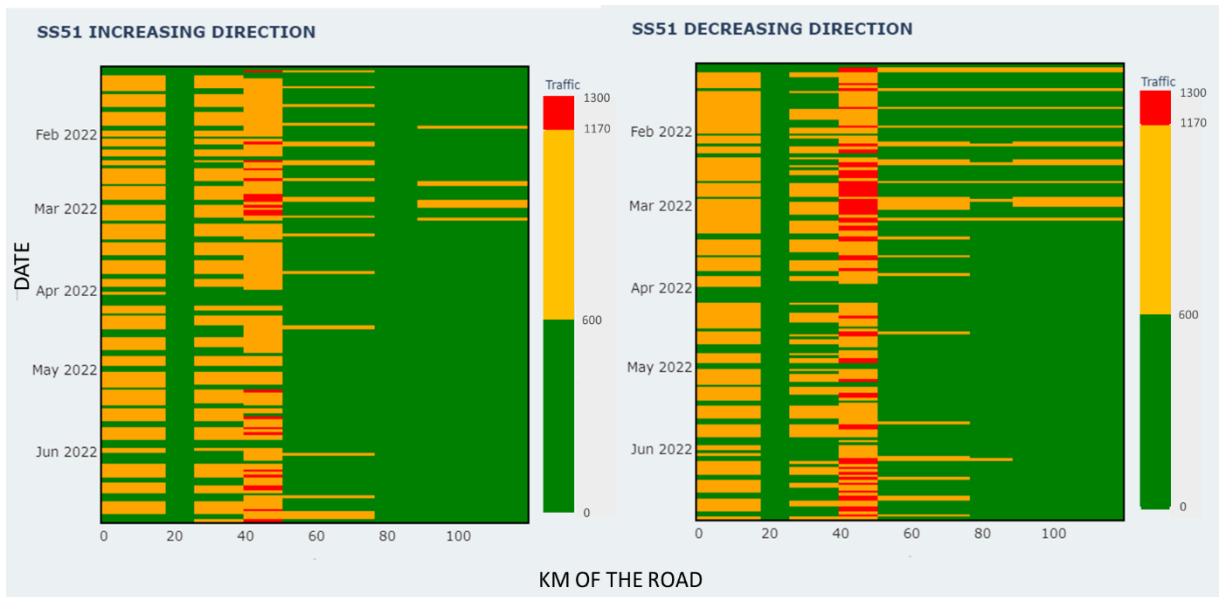
Figure 5. 4: Road Occupancy level representation of SS51 highway
