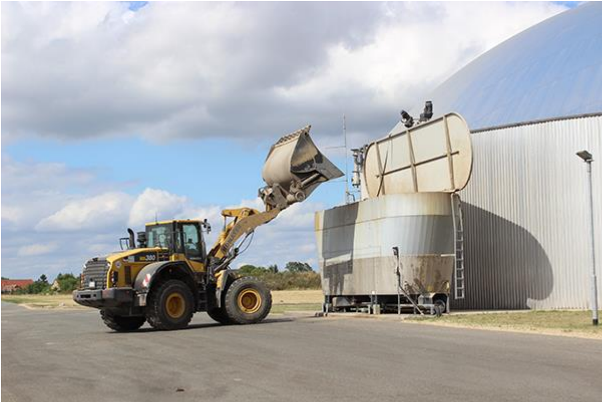
Figure 4.2.2 Biomass substrate loading area. The plant receives 70,000tonnes per year
