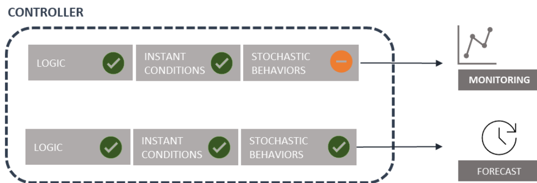
Figure 3.10: Alignment conditions that the controller must satisfy to perform the two services.
