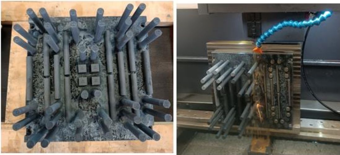
Figure 32: Steelplate after stress relief during EDM cut
