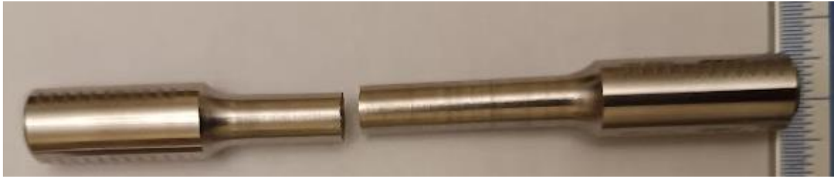
Figure 45: broken H900 specimen
