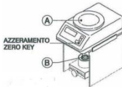
Figure 58: balance used in density measurements
