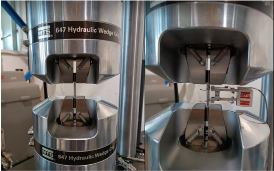
Figure 36: Tensile test and extensometer
