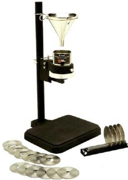
Figure 20: equipment for flowability test [9]
