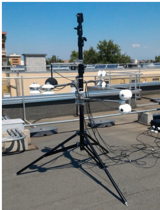
Figure 2. 2. Wires connecting the net radiometers and the datalogger must avoid interferences with the measurements of the radiometers themselves.
