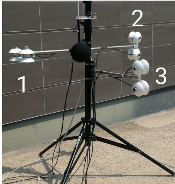
Figure 2. 7. Disposition of the net radiometers near a vertical/horizontal surface.
