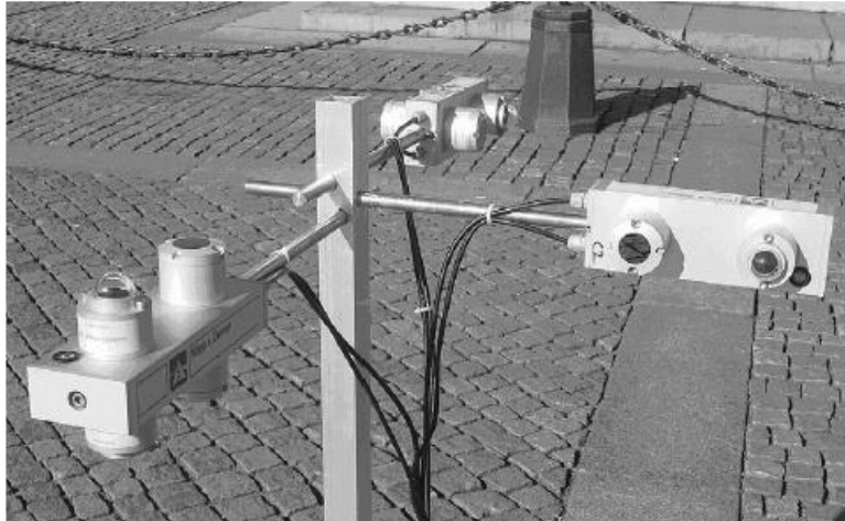
Figure 1. 2 Instruments setup for measuring short-wave and long-wave radiation, using pyranometers and pyrgeometers (Thorsson et al. 2007).
