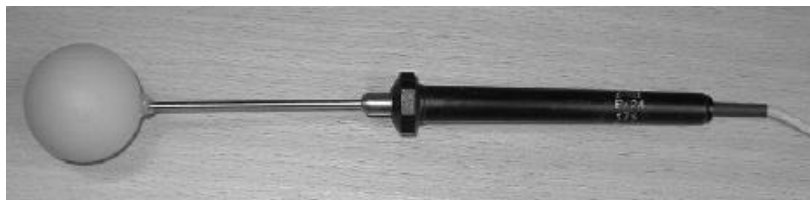
Figure 1. 3. Globe thermometer consisting of a flat grey 40 mm celluloid table tennis ball around a Pt100 temperature probe (Thorsson et al. 2007)
