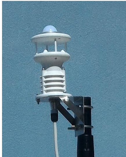
Figure 2. 10. All-in-one sensor able to measure wind velocity and direction, air temperature, solar radiation, air humidity and pressure.
