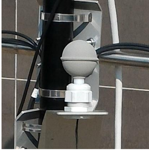
Figure 2. 9. Grey-painted globe thermometer.
