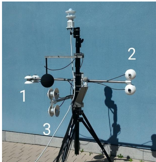
Figure 2. 1. Disposition and numbering of the three net radiometers.
