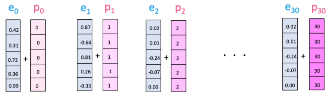
Figure 4: Diagram showing that inserting the token positions in the vector does not work because it causes the values to grow excessively.
