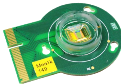
Figure 2. 2. Microelectrode array packaged IC [30]. On the left side of the chip, power and digital interfaces are visible. Neurons can be cultured on top of the fabricated IC.
