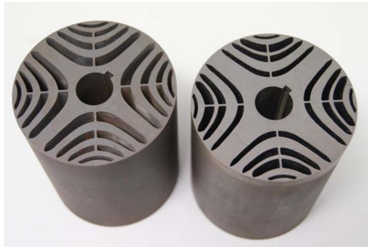
Fig. 5.14 Initial rotor design (right side) and optimized rotor design (left side).
