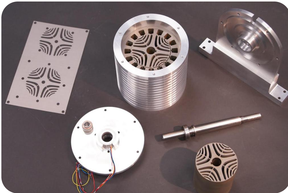
Fig. 5.2 Laminations and the different constituents of the initial SynRM design prototype, M330-35A laminations are used for the prototype.
