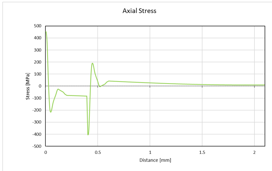
Figure 52_ Representation of the obtained axial stress profile after addition of the 40 th layer
