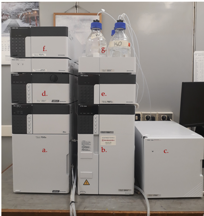
Figure 3.6: HPLC apparatus used in this work: the autosampler (a); oven and columns (b); the fraction collector (c); the pump system (d); the photodiode array spectrometer (e); the controller (f); solvent tray (g)
